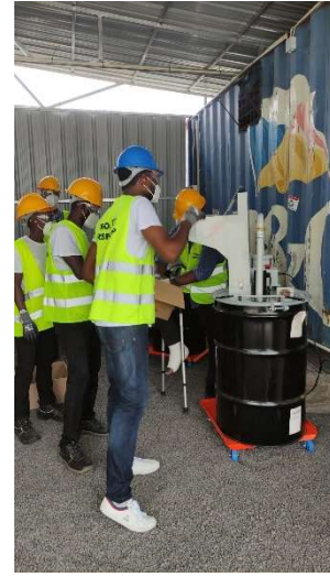
Fig. 7: Employees responsible for crushing lamps and producing glass sand.
