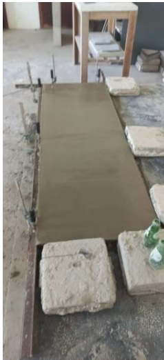
Fig. 5: Manufacturing process for concrete benches with glass sand.
